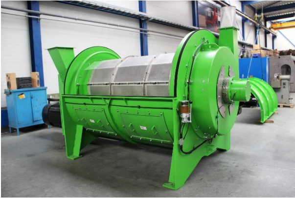
Figure 52. Opened dry washer for plastic reprocessing (source B+B ).
