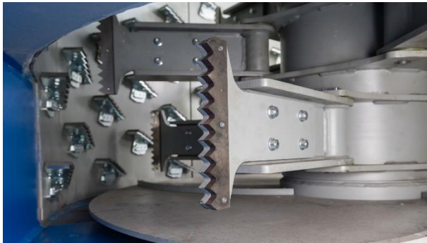
Figure 50. Close-up of the rotor-stator setup of a delabeler (source: Stadler ).
