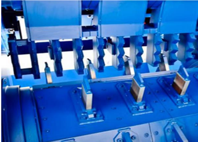
Figure 40. Close-up of a single-shaft bag opener (source: MSW Sorting ).
