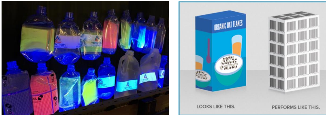
Figure 65. Left: Example of packaging with fluorescent marker as tracer. Right: Example of a readable code (digital watermark) on the packaging surface as tracer.
