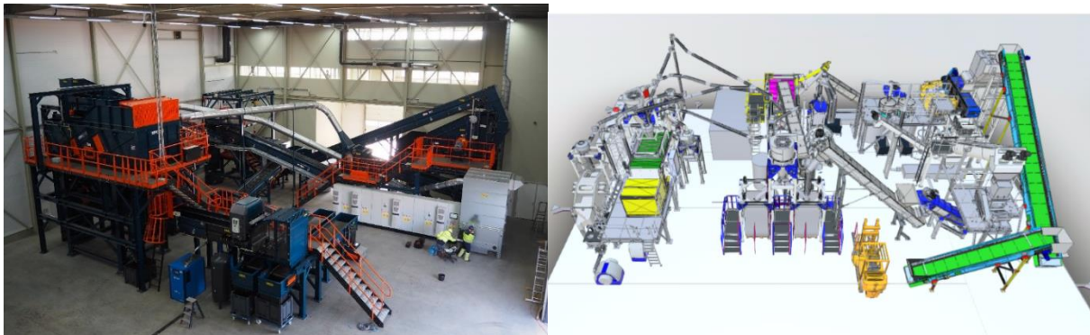
Figure 1. Sorting line (left) and schematic representation of recycling line (right) at NTCP.
