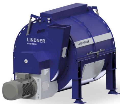
Figure 58. Mechanical dryer for plastic reprocessing (source Lindner Washtech ).
